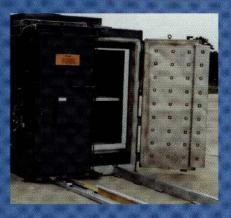
Steelman oven tracks are built in a hinged assembly which allows the doors to be opened or closed over the tracks. Other manufacturers' designs require the operator to completely remove and replace tracks during loading and unloading procedures
